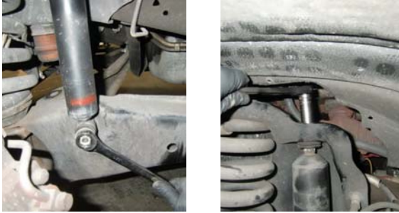
Unbolt the bottom of the shock, then the top.
