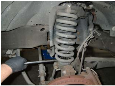
Remove the bottom nut from inside the front coil.
