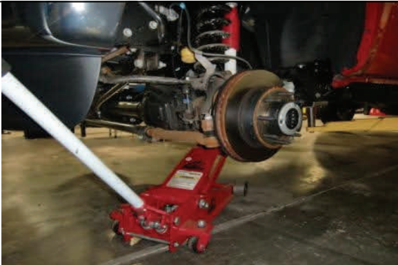
Support front axle with floor jack(s).
