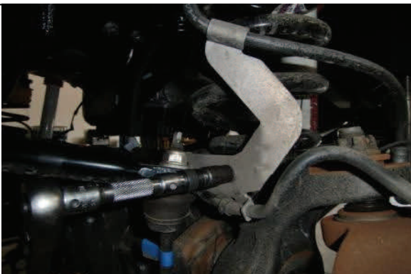
Disconnect brake line support bracket
