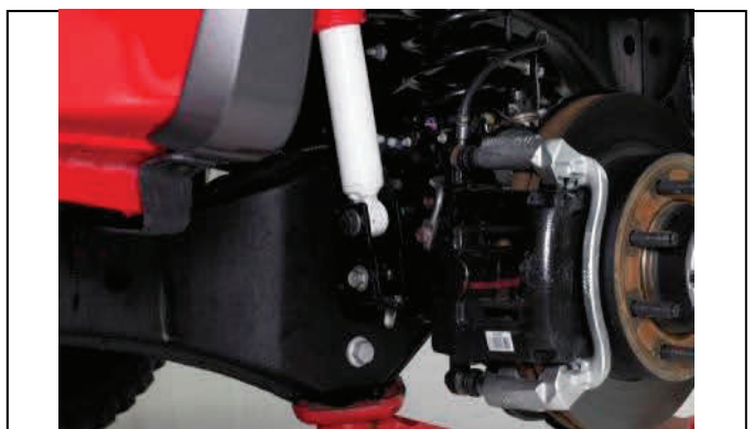
Install and tighten lower shock extension bracket and shock
