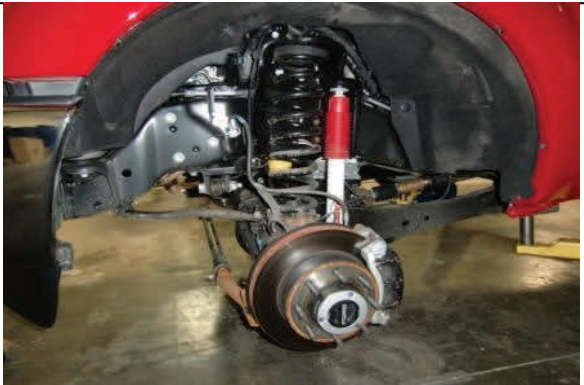
Remove front wheels and tires.
