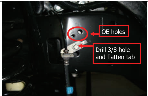
Shown, pass. side new 3/8 brake line hole location.
