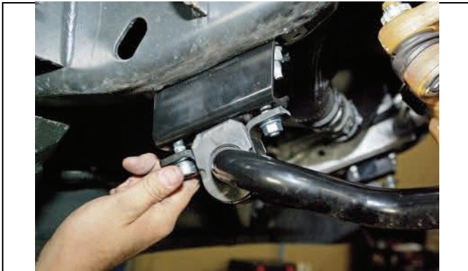
Raise sway bar and attach with new hardware.
