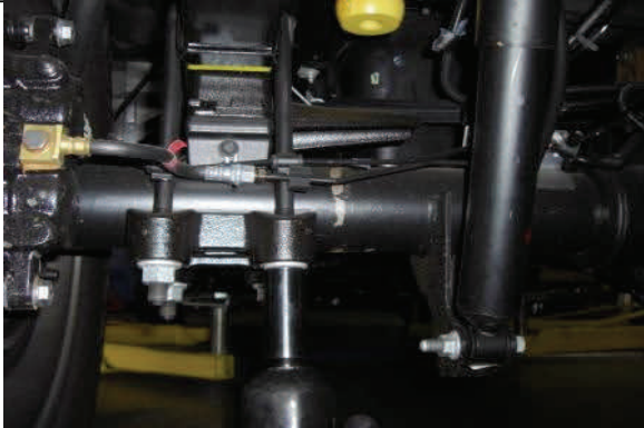
Remove U-bolt nuts and axle mounting plate.
