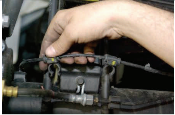
Vehicles with ABS/TC remove clips from U-bolts.
