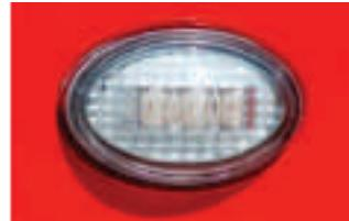
Clean area around fender marker light of dirt and oils. Install the Pure LED Fender Marker light into the existing socket (view below for exceptions). Remove the backing from the tape on the back of the marker light and position light in place.
