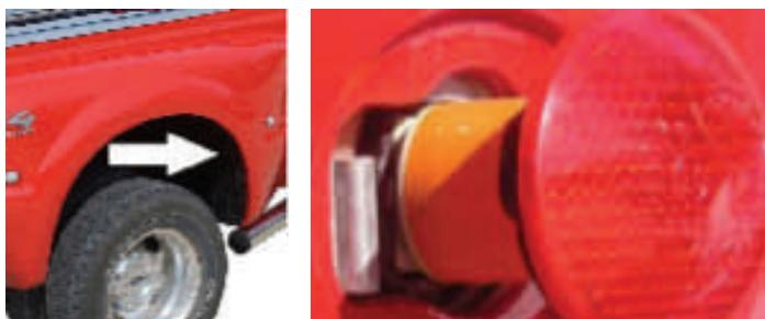
Locate the inner fender plastic and unfasten to allow entry into the fender marker light area. Reach your arm through the inner fender and push the light out.
