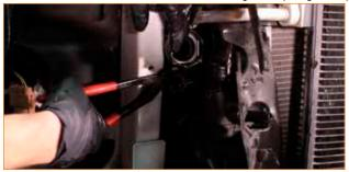
24. Compress the clamp that secures the coolant hose to the driver-side thermostat housing, and remove the hose from the housing. (1x spring clamp)
