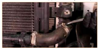
18. Release the two clips from the quick-disconnect fittings on the crossover pipe. Disconnect the upper hose from the crossover pipe by pushing it back, then release the fitting from the thermostat housing by pulling upward. There may be residual coolant inside the system, so keep your bucket handy to capture any spills.
