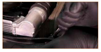
**10.** Disconnect the electrical harness from the horn assembly.
