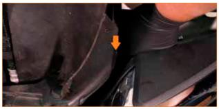
**07.** Release the tree-clip that secures the bottom of the rubber shroud. Do this on both sides. (2x tree-clips)
