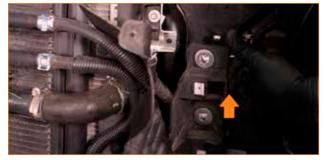
Remove the two bolts that secure the transmission cooler to the radiator support. Allow the cooler to droop over the crossover pipe. (2x 10mm bolts)
