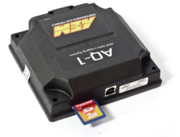
FIGURE 3: AEM AQ-1 Data Logging System.
