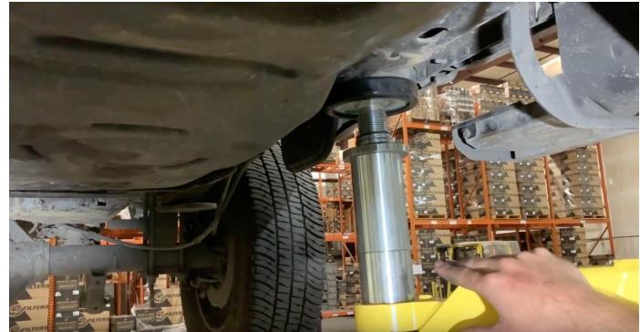
truck is lowered or has running boards you may have to use a jack to get the S&B Tank in position.
