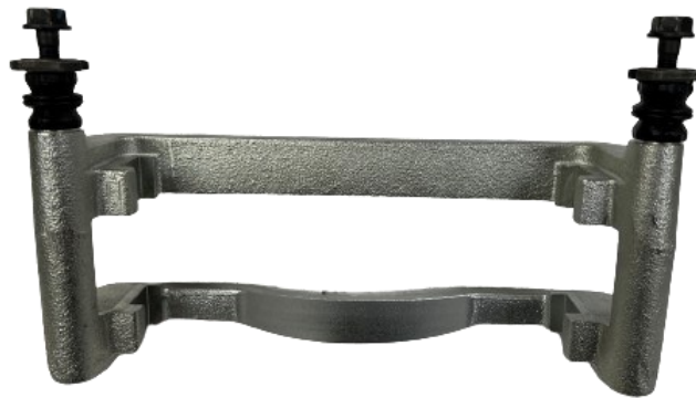
INSTALL THE PREPPED SLIDING PINS INTO THE BIG CLAW ANCHOR BRACKET
