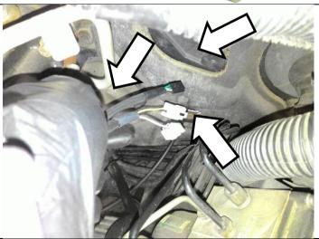
Route the two white plugs behind the dash to the shift lever connectors. Connect the harness to the shift lever and to the trucks stock wiring harness.
