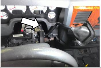
Follow the twisted black wire from the stock shift lever under the column to the two pin connector. Disconnect the plug and remove the push in retainer.
