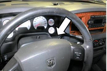
Install wire ties under the dash to support the harness to the existing vehicle wire harnesses.
