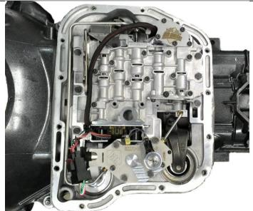
Unplug the transmission wiring harness from the governor solenoid by releasing the tab on the bottom side.
