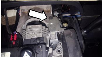
Connect the shifter linkage by pushing the socket back onto the ball.
