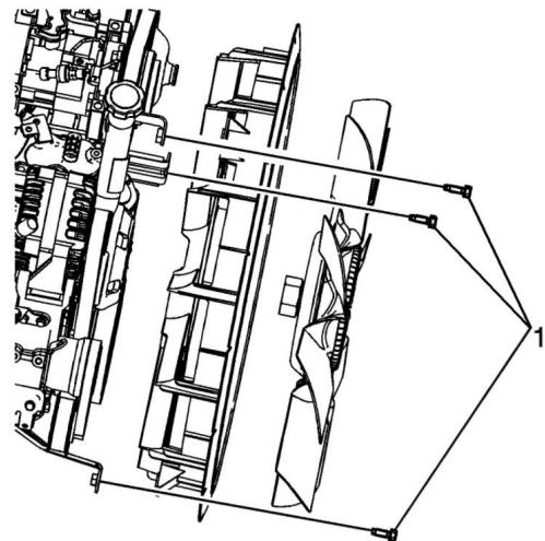
4. Position the engine cooling fan shroud forward to the radiator.
