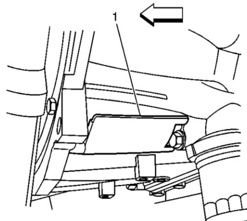
24.If reusing torque converter bolts, clean the bolt threads and apply LOCTITE 242 or equivalent to the threads prior to installation.
