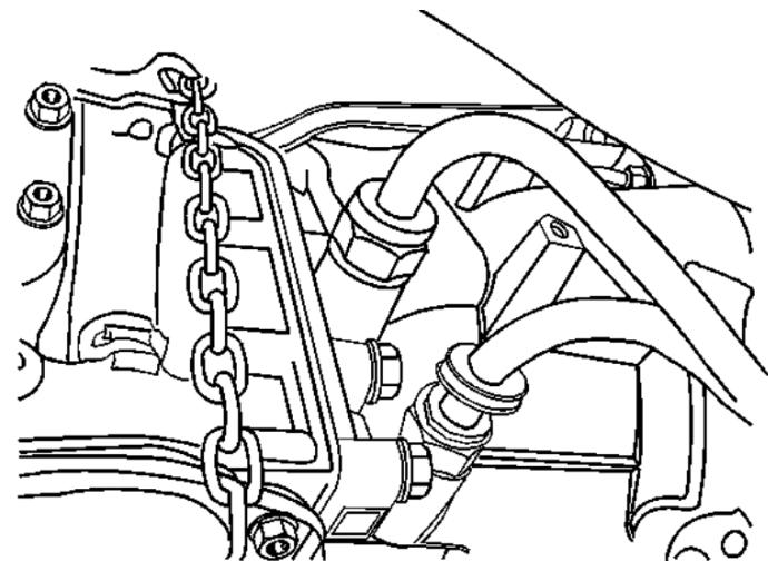
12. Position exhaust hanger and install the bolts and tighten to 12Nm (106 lb-in).
