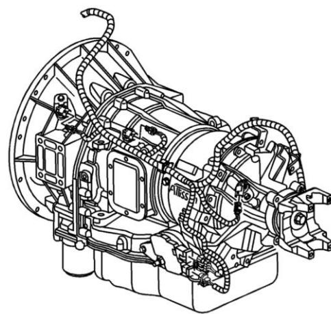
18. Disconnect the transmission main electrical connector. J 44257 tool may be used for ease.
