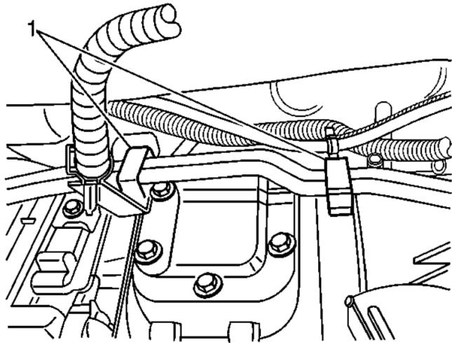
16. Remove the fuel line bracket nut from the converter housing stud.
