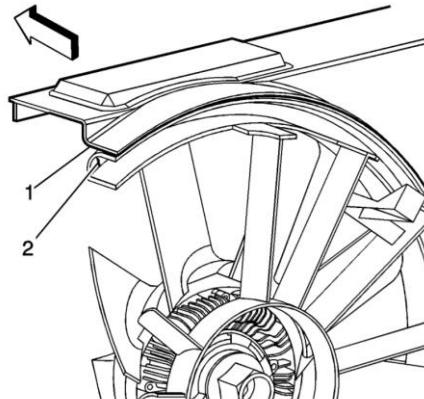
32. Fully tighten the 3 engine cooling fan shroud bolts and tighten to 8Nm (7 lb-in).
