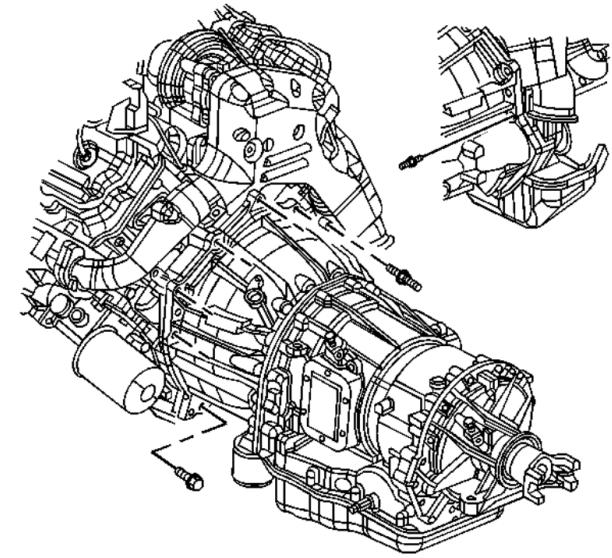
7. Install the wire harness/vent tube bracket and nut to the converter housing stud. Tighten the nut to 18Nm (13ftlb).
