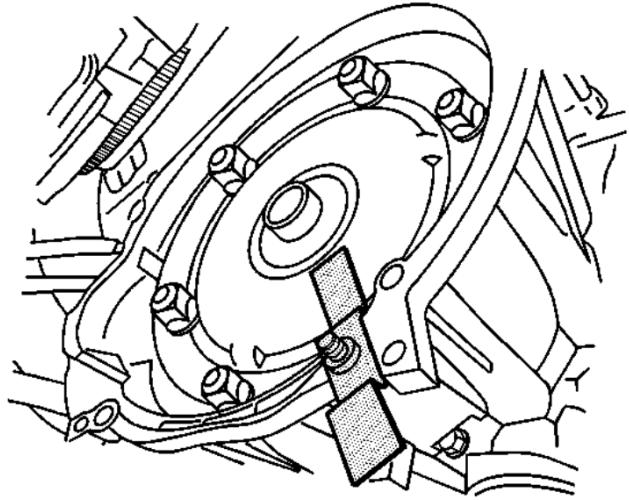
5. Align the transmission with the engine using the alignment dowels located at the rear of the engine.
