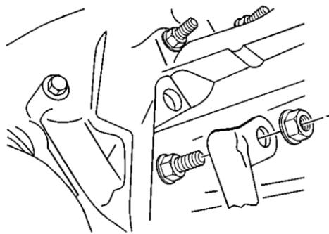
18. Install the fuel line retainer and bolts to the left side of the transmission and tighten to 2.2Nm (22 lb-in).
