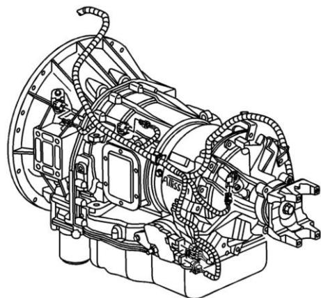
17. Install the fuel line bracket and nut to the transmission converter housing stud. Tighten the nut to 18Nm (13ftlb).
