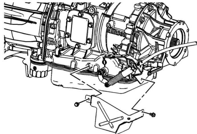
23. Remove the access hole cover on the converter housing in order to rotate the converter and align the first torque converter bolt.
