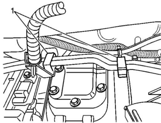
20. Install the range selector cable end to the transmission range selector lever stud.
