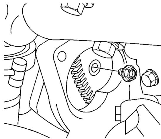
10. Remove the range selector cable heat shield bolts.
