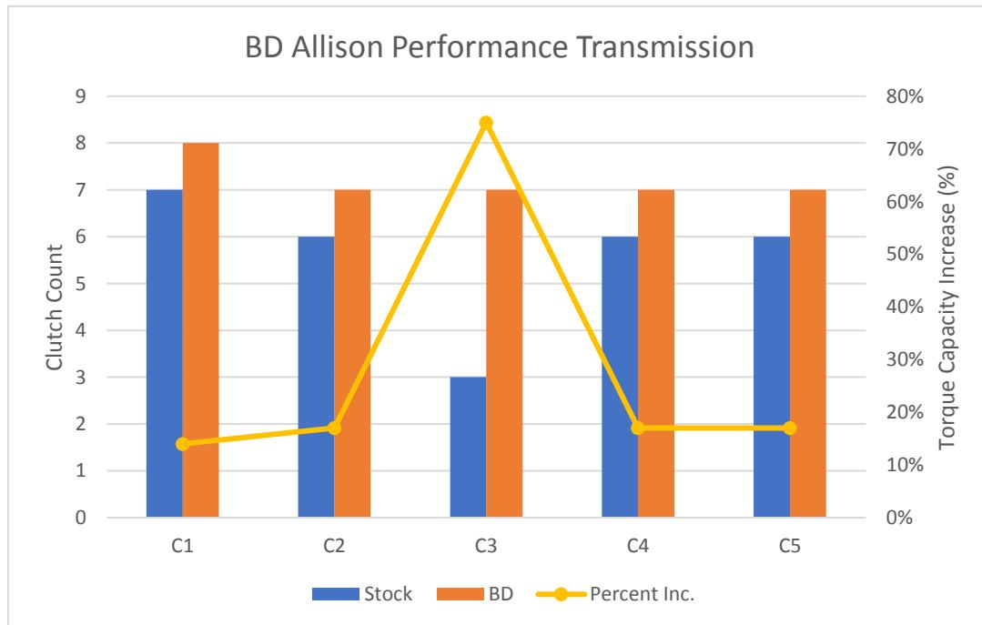
The main failure in Allison Transmissions is the C3 clutch, in which BD has increased the clutch count by 4, increasing the torque capacity by 75%. The chart above shows the increase and improvements in each of the clutch packs in the BD Allison Transmission over the stock.
