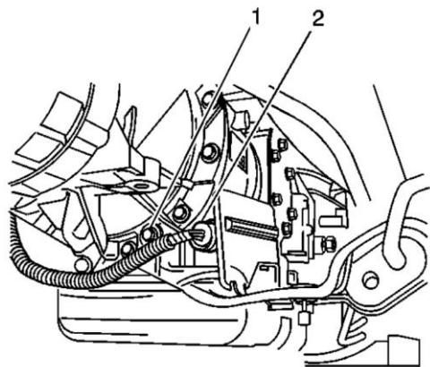
16. Connect the electrical connects on the transmission and transfer case.
