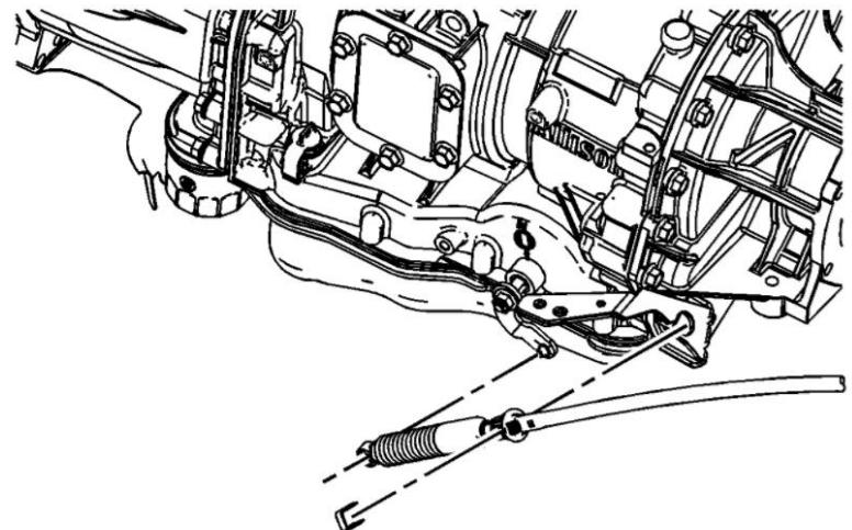
21. Install the range selector cable heat shield.
