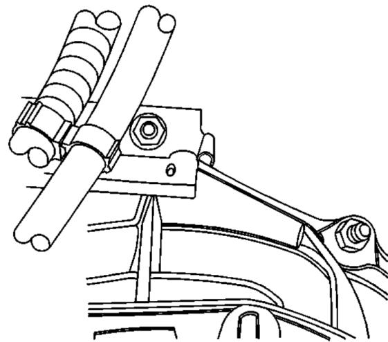
10. Remove the safety chain from around the transmission.
