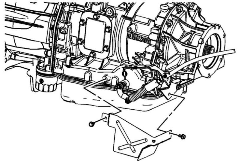
12. Remove the range selector cable end from the transmission range selector lever stud.
