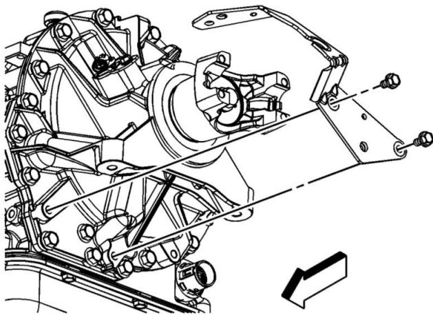
2. Install the J 21366 strap to the converter housing in order to keep torque converter from sliding off the turbine shaft.
