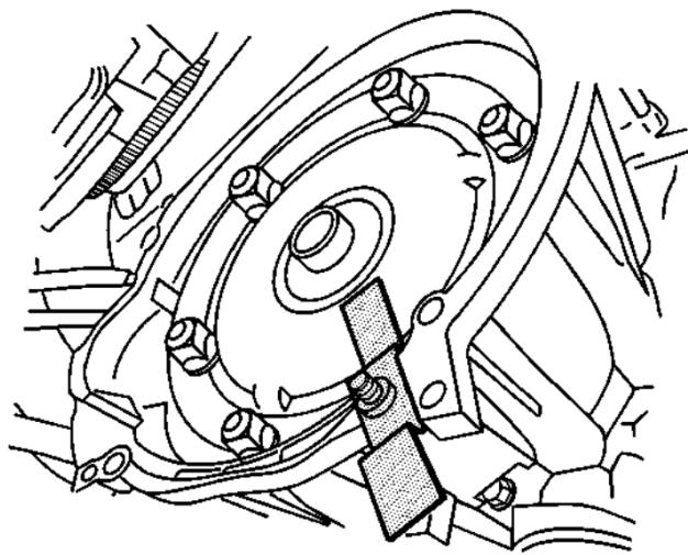
35. Remove the shift cable bracket and bolts to the transmission.
