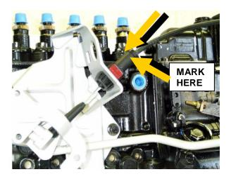
**<u>NOTE:</u>** Disconnecting the cable from the support bracket and the throttle lever is a difficult task; it may be easier to adjust without removing cable.
