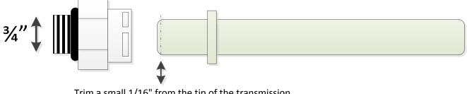
Trim a small 1/16" from the tip of the transmission cooler line. Leave no sharp edges.
