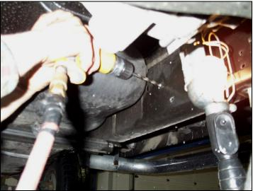
Using a 5/16" drill bit, drill pilot holes for thread cutting mounting bolts.
