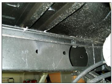
Locate and clean a spot to mount the filter housing along the left hand (driver side) frame rail.
