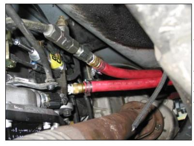
Measure and cut a section of the blue transmission filter hose supplied and install onto the barb fitting at the "IN" port of the filter head and secure it tightly with hose clamps. Install the other end of the hose onto the barb fitting attached to the return line from the cooler and secure tightly with hose clamps.
