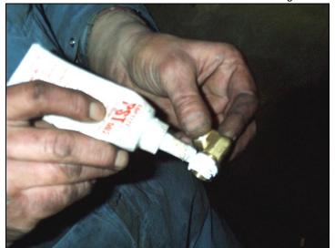
Install the two ½" hose x ½" NPT barbed fittings (1604047) into the 90° ORB fittings (1604046) using some pipe sealing compound or tape to the threads of the brass barb fittings only.
