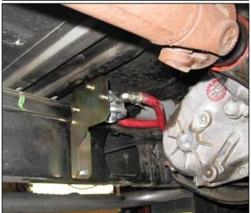
Position the filter mounting bracket and install the 2 thread cutting mounting bolts using the flat washers supplied.
