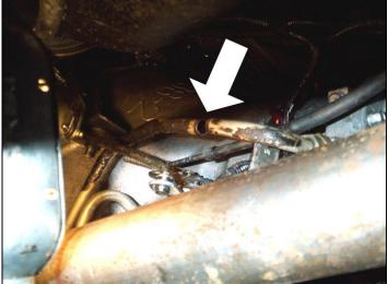
Using a small pipe cutter, cut the line approximately 6" from the bend. NOTE: You may want to use the drain pan to capture any spilled fluid.
