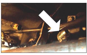
Install the straight 1/4NPT-JIC (1604048M) fitting into the open port on the transmission using pipe sealant on the threads. Thread the fitting in finger tight, and then turn once more with a wrench. Do not over torque as you will damage the case.
