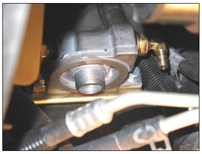
Position the filter head on the filter mount and secure using the 3 mounting bolts and washers supplied. Leave the filter off at this point as it will be installed later.
