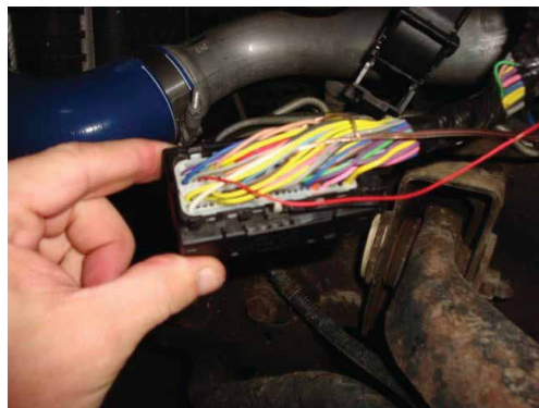
STEP 5 INSERT NEW PINS/WIRES *REVERSE PROCEDURES WHEN FINISHED*
