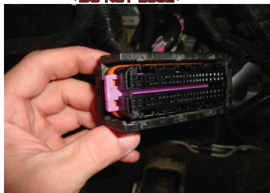
STEP 5 INSERT NEW PINS/WIRES *REVERSE PROCEDURES WHEN FINISHED*
