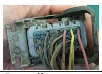
STEP 11 INSERT PIN & WIRES TO LATCH, REINSTALL PIN LOCK
