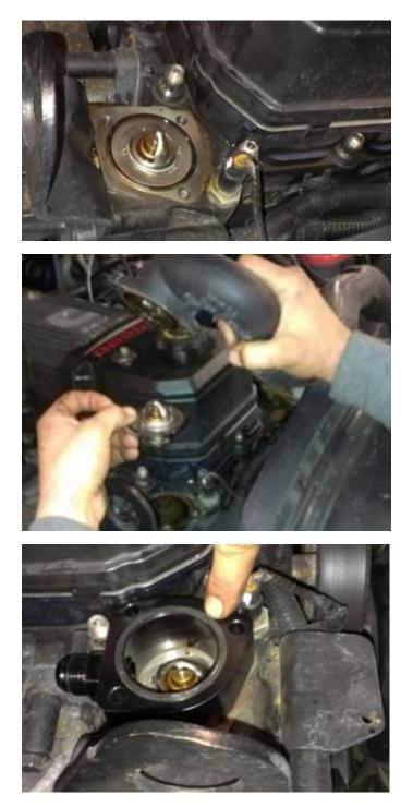
STEP 6: Place the stock thermostat housing over the thermostat riser block. Using the supplied M6 flange head bolts (item 5), tighten the bolts to 89 in-lbs.
