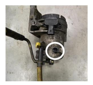
10. Install the WIF sensor in the bottom of the fuel distribution block.
