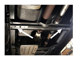
STEP 4: Secure the tank with a lift or jack to lower the tank down to the ground.
