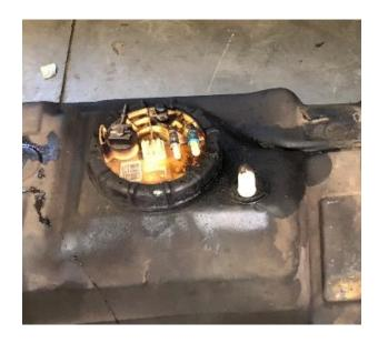
Using a strap wrench, or MATCO tool #FTR730, rotate the sending unit's retaining ring (OE P/N: 52005389) counterclockwise. MATCO tool shown at right for reference. Remove the retaining ring and remove the sending unit assembly from the tank. Have a bucket nearby to catch fuel from the OE sending unit when removed.
