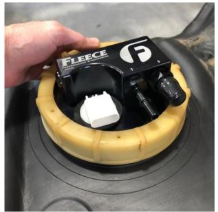
STEP 13: Remove the protective shipping caps from the fittings and install the new fuel line locking tab that is included in your kit onto the return side fitting.
