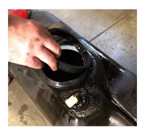
STEP 9: Once the area is clean, install the new seal ring included in the kit into the fuel tank.
