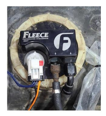
Clean the mechanical fuel pump mounting surface and install the fuel pump block off plate included in the kit.
