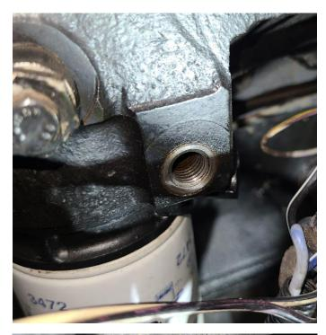
STEP 5: Install the new banjo fitting, 12mm banjo bolt and two, 12mm copper crush washers included in the kit onto the open port on the fuel filter housing.
