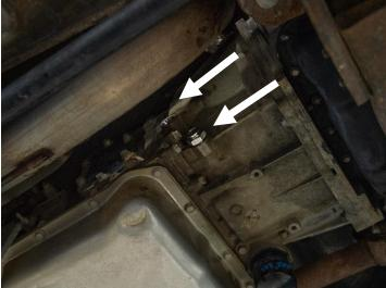
With the OE transmission lines removed from the truck, use a  $1 \frac{1}{8}$  back up wrench and  $1 \frac{1}{4}$  socket or wrench to remove the factory fittings from each side of the transmission cooler.
