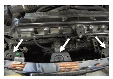
Remove the front grill retention bolts located along the top of the grill.
