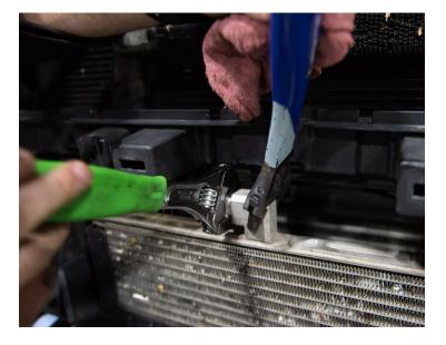
Install two of the 7/8"-14 O-ring to -10AN fittings into the left and right side ports of the oil cooler.
