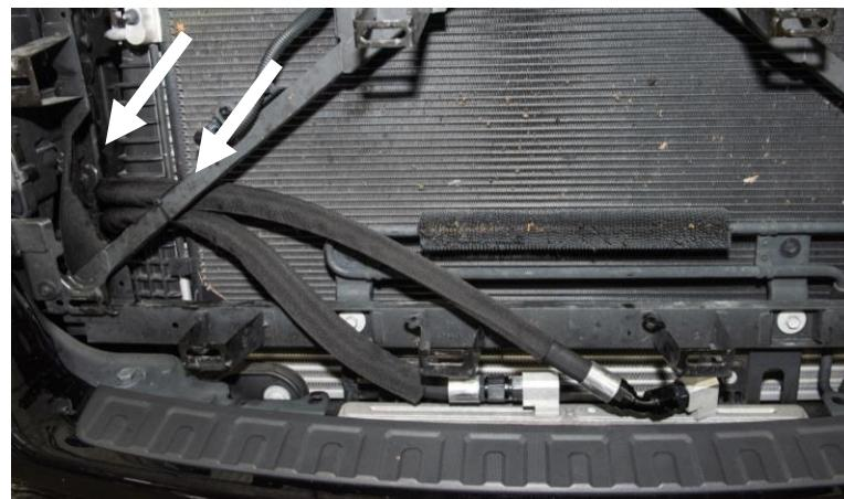
The shortest line is routed from the left side (passenger side) of transmission cooler to the top-side radiator fitting.
