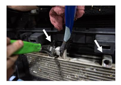
Install one of the 7/8"-14 O-ring to -10AN fittings into the left side port of the oil cooler.
