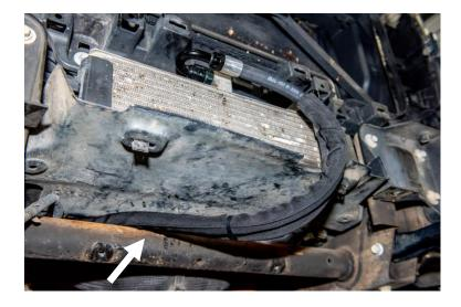
Use the double hose clamps provided in the kit to secure the hoses together.
