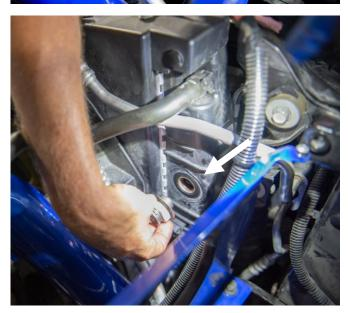
Install the two fittings into the radiator, removing and replacing one fitting at a time.
