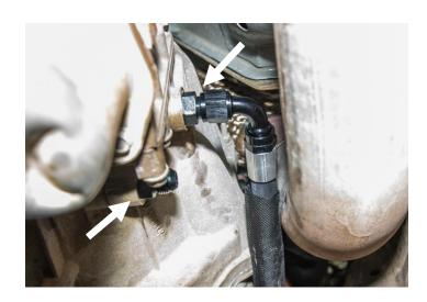
Mark and trim the plastic shroud below the transmission cooler approximately 3" to allow for additional room to route the new transmission lines.
