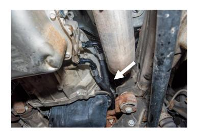
Route the long and short length lines over the main chassis members and suspension anti-roll bar.
