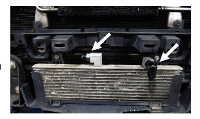
Assemble the large flat washers onto two of the 7/8"-14 O-ring to -10AN fittings.
