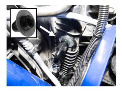
Remove the two OE fittings from the transmission using a 1 ½" socket or wrench.
