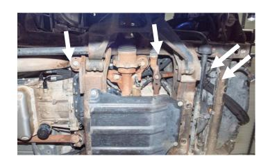
The short length hose is routed from the transmission "TO COOLER" to the bottom-side radiator fitting. The 45 degree fitting is utilized on the radiator side, aligned slightly downward and toward the center of the chassis.
