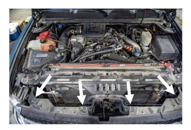
Using a long pry bar, release the lower retaining clips for the front grill.
