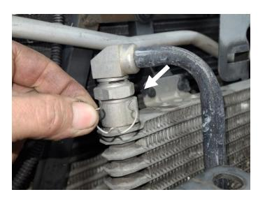
With the OE transmission lines removed from the truck, use a 1 1/8" back up wrench and 1 1/4" socket or wrench to remove the factory fittings from each side of the transmission cooler.
