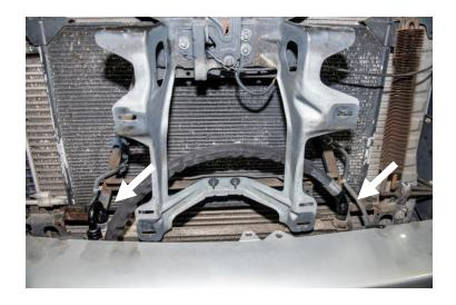
Assemble the large flat washers onto two of the 7/8"-14 O-ring to -10AN fittings.
