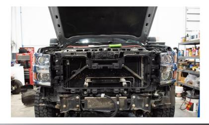
Remove the lower engine shroud.
