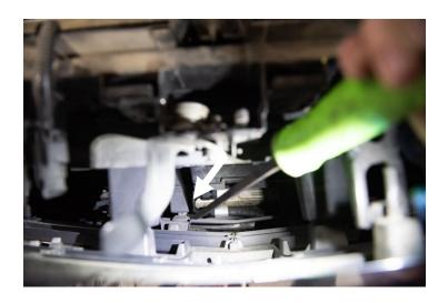
Remove the front grill. Next remove the front bumper by removing the upper retaining bolts with an 18mm socket.
