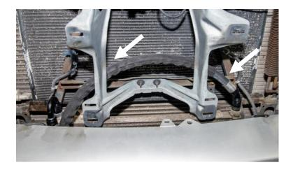
The medium length hose (with the 180 degree fitting) is routed to the left (passenger side) of the transmission cooler. Use the fir tree wire tie to secure the longest hose to the cooler bracket at the hole location shown at right.
