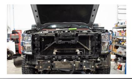
Remove the lower engine shroud.
