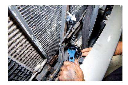
Route the lines over the top of the chassis cross-tube. Use the double hose clamps provided in the kit to secure the hoses together.
