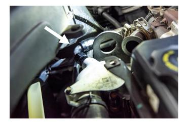
STEP 21: Reinstall the heat shield over the coolant bypass elbow.
