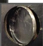
STEP 4: With the freeze plug removed, use a Scotch-Brite<sup>™</sup> pad and a degreasing solution to **thoroughly** clean the block surface area from the head down to the rear cover, as well as the bore where the freeze plug was previously installed. Be sure to remove all dirt and foreign debris to allow the coolant bypass thermostat housing to fully seat. If the inner bore where the freeze plug was seated is not thoroughly clean, the O-ring on the coolant bypass housing will not properly seal.
