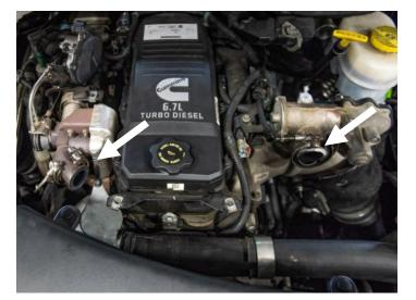
STEP 15: Remove the two, 8mm bolts that retain the heat shield to the top of the cooler elbow. Remove the heat shield.
