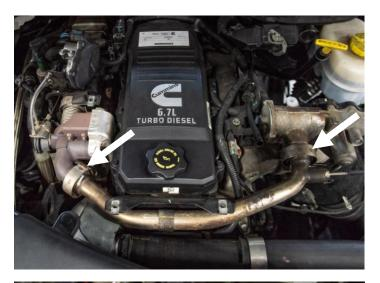
STEP 13: Remove the 8 mm bolt that retains the cross over tube at the front of the engine.
