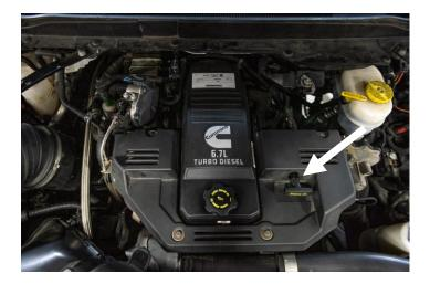
STEP 10: Remove the 4, 8 mm bolts that retain the engine shroud and remove the engine shroud.
