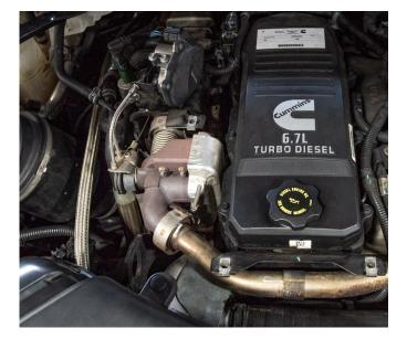
STEP 24: Plug in the EGR temp sensor and install the upper engine shroud. Insert the dipstick. Ensure that the coolant drain plug has been reinstalled in the radiator and proceed to re-fill the coolant system. Re-use or replace coolant as necessary to properly fill the system with clean fluid.
