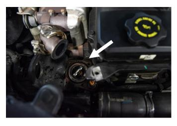
into the same location as the factory coolant elbow. Install the three new M6 bolts included in the kit that retain the coolant elbow to the cylinder head. Reinstall the coolant hose and clamp.
