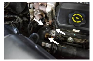
STEP 18: Remove the thermostat. Inspect it for wear and proper function. With a Scotch-Brite<sup>™</sup> pad and degreasing solution, thoroughly clean the sealing surface of the stock thermostat and thermostat housing. Be sure to remove any foreign debris and reinstall the OE thermostat.
