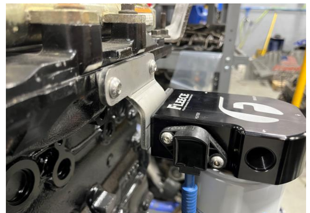
MY 2010+; mounted downwards directly to head
