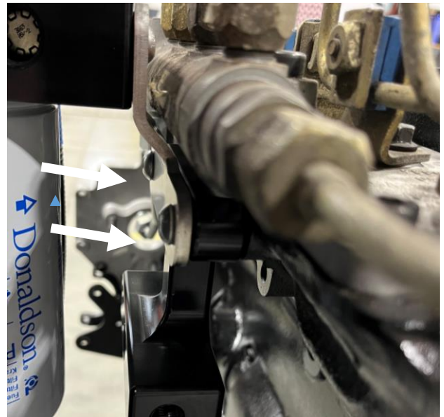
MY 2003-2009; mounted over fuel filter delete
