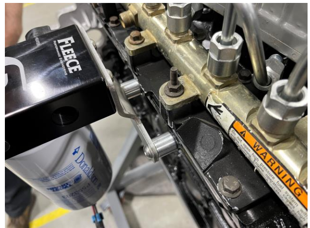
MY 2010+; mounted upward with spacers
