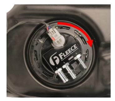
Remove the hex cap to allow for pump return fuel to feed the bucket
