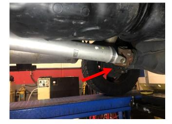
STEP 4: Support the fuel tank with a lift jack. Loosen the front and rear fuel tank straps using a 15mm deep socket. Remove the front strap first, and leave the rear strap loose and attached at this time. Lowering the front of the fuel tank downward will allow access to unplug the sending unit and remove the fuel line quick disconnects and vent line.
