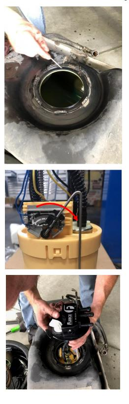
STEP 11: Reinstall the original retaining ring using your hammer and punch by rotating it clockwise to the fully engaged position.
