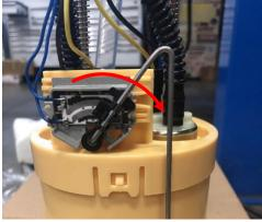
STEP 10: Install the SureFlo assembly into the tank, use caution with the float arm and do not over-rotate the pump once installed.
