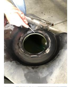
STEP 9: Install the fuel level float arm onto the SureFlo assembly by gently clipping the arm into the fuel level sensor.
