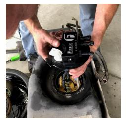
NOTE: Use caution when installing the SureFlo to not damage the float arm. Do not rotate the pump once it is installed in the tank, you may damage the float arm or sending unit – align it before you place it into the tank.
