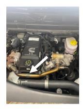
STEP 2: Remove the cross over tube from the EGR to the intake horn; Loosen the V-band clamp at either end of the cross over tube. Remove the one bolt that retains the cross over tube to the cylinder head located at the front of the engine.
