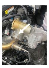
STEP 3: Remove the intake horn; Remove the 6 bolts that retain the intake horn to the cylinder head intake shelf. Remove the 1 bolt that retains the dipstick tube to the intake horn. Remove the T-Bolt clamp from the intake tube.
