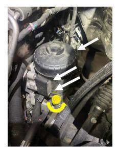
**STEP 8:** Remove the two zip ties retaining the electrical harness to the fuel filter base.
