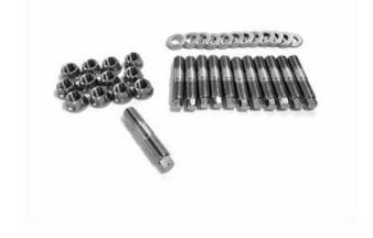
Use a small amount of oil or anti-seize on the threaded side of the stud that will be in the head. Run each stud in by hand into the head. Gently snug each stud to the bottom of the bore. DO NOT OVERTIGHTEN.
