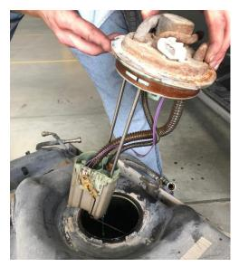
STEP 8: Clean all debris from around the o-ring groove and tank sealing surface. Place your <u>new</u> o-ring supplied in the kit for the PowerFlo lift pump onto the top of the tank.
