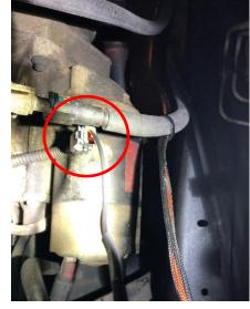
STEP 19: From the driver's side rear wheel-well, connect the electrical wiring harness to the PowerFlo lift pump connector.
