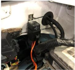
STEP 17: BATTERY CONNECTIONS Run the orange fused line to the positive (+) terminal of the battery. Run the black line to the negative (-) terminal of the battery.
