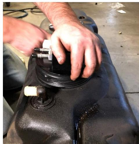
STEP 13: Reinstall the retaining ring using your hammer and punch or a strap wrench by rotating it clockwise to the fully engaged position. Ensure proper orientation of the pump and fitting by matching the orientation of the original sending unit.
