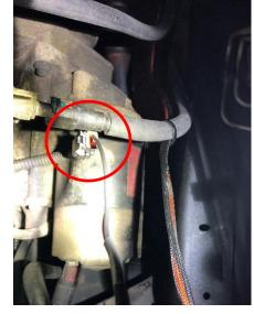
STEP 20: From the driver's side rear wheel-well, connect the electrical wiring harness to the PowerFlo lift pump connector.
