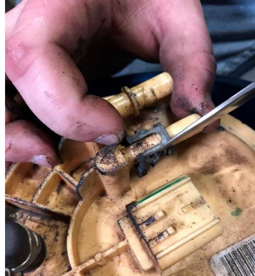
**STEP 9:** Remove the gasket from the tank.
