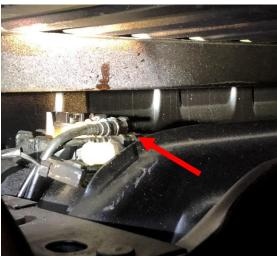
STEP 3: Remove the cross-member located at the front of the fuel tank. There will be 4, 15mm bolts to remove.
