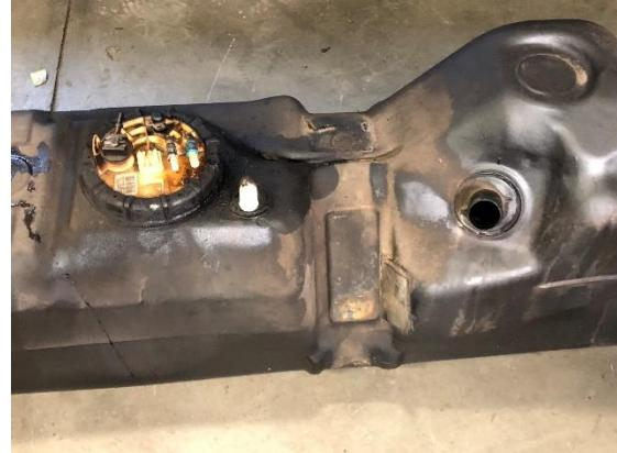
Using a strap wrench, or hammer along with a chisel or drift, rotate the sending unit's retaining ring counter clockwise.
