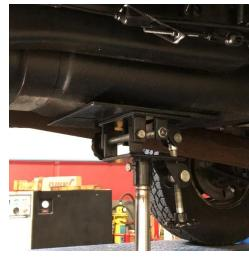
STEP 5: Remove 15 mm nuts that retain the fuel tank hanger brackets at the front and rear of the tank. Remove the hangers.
