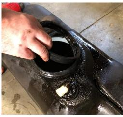
STEP 10: Install the new gasket included in the kit onto the PowerFlo pump, installing it onto the top of the sending unit by sliding it up from the bottom. Clean the retaining ring of debris and prepare it for re-use onto the new PowerFlo pump.
