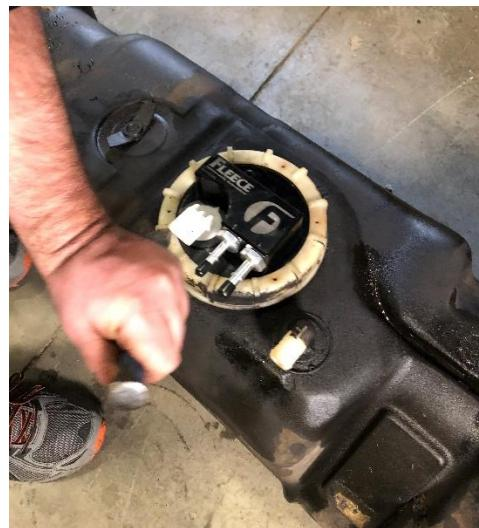
*NOTE: Use caution when installing the pump to not damage the float arm. DO NOT rotate the pump once installed in the tank, you may damage the float arm or sending unit – align the pump before you place it into the tank.*
