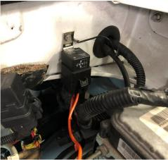
STEP 18: BATTERY CONNECTIONS Run the orange fused line to the positive (+) terminal of the battery. Run the black line to the negative (-) terminal of the battery.
