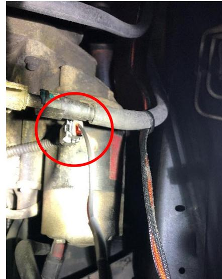
STEP 20: From the driver's side rear wheel-well, connect the electrical wiring harness to the PowerFlo lift pump connector.
