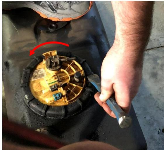
Remove the retaining ring and remove the sending unit assembly from the tank. Have a bucket nearby to catch fuel from the OE unit when removed.
