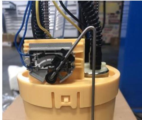
STEP 12: Install the PowerFlo pump assembly into the tank. Check the gasket for proper seating. Gently work the seal around the ID of the bore to fully seat the seal.
