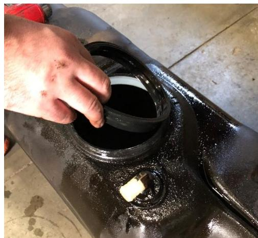
**STEP 10:** Install the new gasket included in the kit onto the PowerFlo pump, installing it onto the top of the sending unit by sliding it up from the bottom. Clean the retaining ring of debris and prepare it for re-use onto the new PowerFlo pump.
