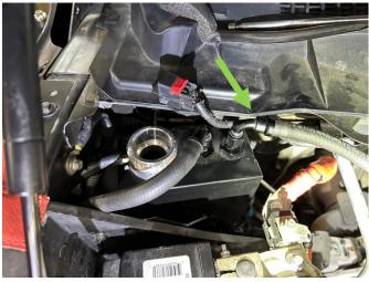
STEP 9: Using the -6AN 90 deg pushlock fitting included in the kit, attach this to the degas line that was disconnected from the OE coolant tank. It may be necessary to trim a small amount of hose to achieve a uniform routing along the left side of the tank.
