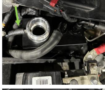
STEP 11: Install the -12AN 90 degree fitting onto one end of the new  $\frac{3}{4}$ " heater hose included in the kit. Secure the hose to the fitting with one of the hose clamps included in the kit. Slide the heat wrap removed from the OE coolant hose over the new  $\frac{3}{4}$ " hose.
