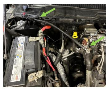
STEP 8: Connect the 90 degree -6AN fitting and hose that routes to the coolant riser pipe to the right side -6AN fitting on the coolant tank.
