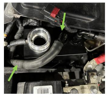
STEP 10: Install the overflow vent hose onto the tank and route it down along the left side of the tank.
