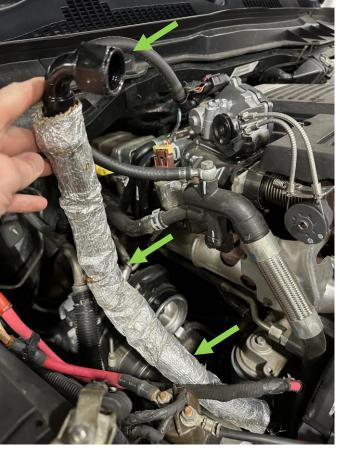
STEP 12: Route the coolant hose and secure it with zip ties to prevent it from making contact with any hot or rotating components.
