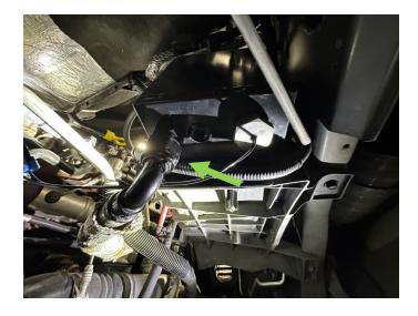
STEP 14: Connect the coolant level sensor to the factory harness that was disconnected during removal of the OF tank.
