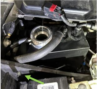
STEP 7: Using the 3/8" hose included with the kit, slide one end onto the banjo fitting on the top of the coolant riser pipe. Secure the hose to the fitting with an included hose clamp. On the other end of the 3/8" hose, insert one of the pushlock 90 degree -6AN fittings.
