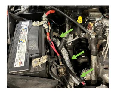
STEP 13: Connect the -12AN 90 deg fitting on the end of the coolant hose to the -12AN connection on the coolant tank.
