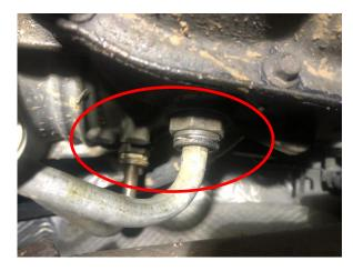
STEP 5: Remove the c-clip retainers at the transmission (2 locations), and release the retaining caps to free the lines from the port.
