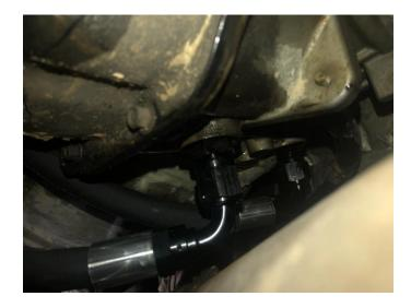
STEP 9: Using four double-hose zip ties (item 4), space them evenly along the length of the cooler lines. Tighten the ties to retain the hoses together.
