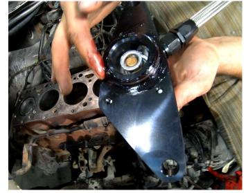
STEP 8: Slide the thermostat housing between the firewall and the back of the engine block. Align the thermostat housing with the original freeze plug hole location and press the housing against the engine to seat the housing. The coolant bypass hose should be oriented towards the passenger side of the vehicle and over the exhaust manifold.
