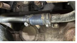
STEP 7: Install the new heater hose and hose clamps and coolant pipe to the heater core connection on the firewall. Use the P-clamp, M8x30mm bolt and ¾" aluminum spacer, to offset the new heater tube from the engine block.
