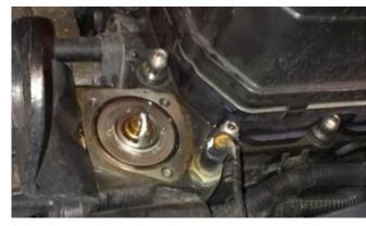
STEP 9: Remove the stock thermostat. Inspect it for wear and proper function. With a Scotch-Brite ™ pad and degreasing solution, thoroughly clean the sealing surface of the stock thermostat and thermostat housing. Be sure to remove any foreign debris, and reinstall the OE thermostat.
