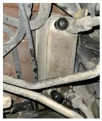
STEP 6: Install the 16mm coolant plug port into the engine block where the barb fitting was removed.
