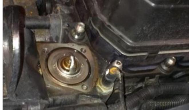
STEP 9: Remove the stock thermostat. Inspect it for wear and proper function. With a Scotch-Brite™ pad and degreasing solution, thoroughly clean the sealing surface of the stock thermostat and thermostat housing. Be sure to remove any foreign debris, and reinstall the OE thermostat.
