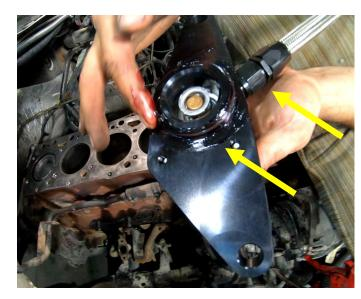
STEP 16: Slide the thermostat housing between the firewall and the back of the engine block. Align the thermostat housing with the original freeze plug hole location and press the housing against the engine to seat the housing. The coolant bypass hose should be oriented towards the passenger side of the vehicle and over the exhaust manifold.
