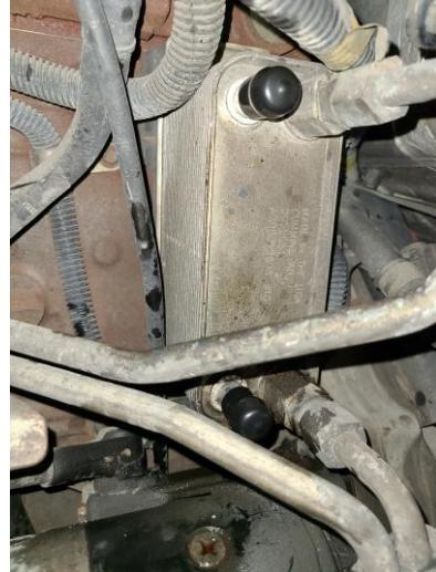
STEP 6: Install the 16mm coolant plug port into the engine block where the barb fitting was removed.
