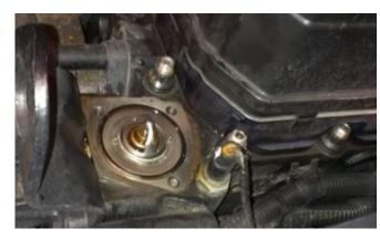
STEP 9: Remove the stock thermostat. Inspect it for wear and proper function. With a Scotch-Brite ™ pad and degreasing solution, thoroughly clean the sealing surface of the stock thermostat and thermostat housing. Be sure to remove any foreign debris, and reinstall the OE thermostat.
