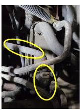
STEP 4: Remove the hose from the transmission heat exchanger that runs to the side of the engine block. Remove the threaded barb fitting from the engine block.
