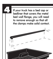
For bed caps, trim only enough of the bed cap edge so the rear (tailgate) clamp contacts the bottom of the metal flange.
