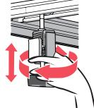
Rotate the body of the clamp up or down to match it's position with the bed rail flange.
