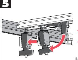
The front (cab) clamp stows in the cover rail. Rotate the clamp down and slide it at an angle towards the bed rail.
