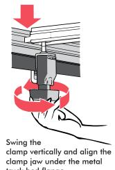
truck bed flange. Tighten the T-handle by hand.
