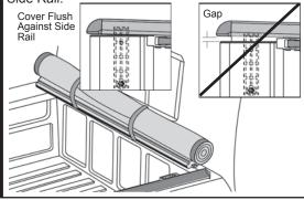
**5** Secure Driver Side Rail to Tonneau Cover Assembly
