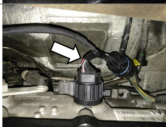
Install supplied zip-ties to support the wiring harness between the engine bay and transmission.
