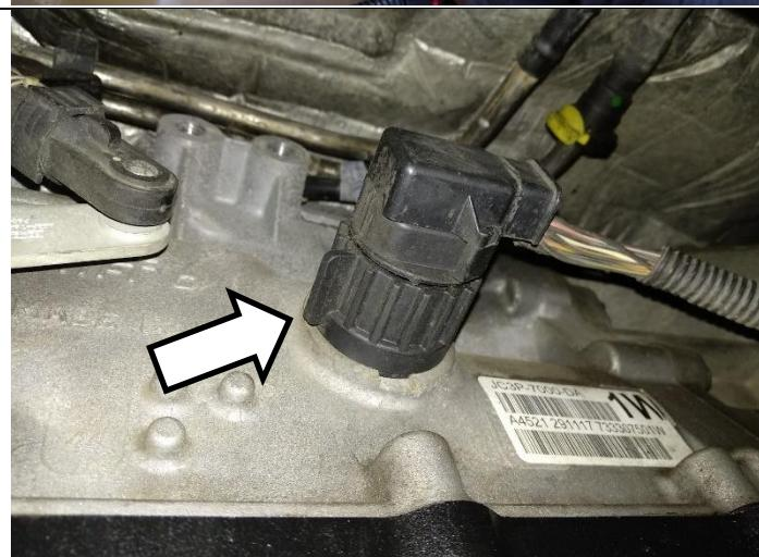
Route the supplied BD harness to the transmission and connect it inline.
