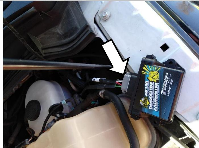
Use the supplied Velcro or use zip-ties to mount the module in the desired location.
