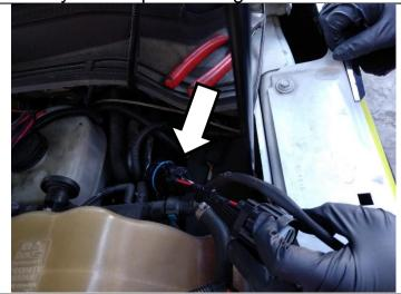
Under the truck, locate the transmission connector. Rotate the lock ring counter clockwise to release it.
