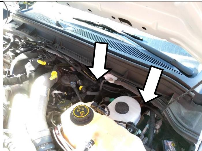
Plug the module into the wiring harness and tie up extra wire slack.
