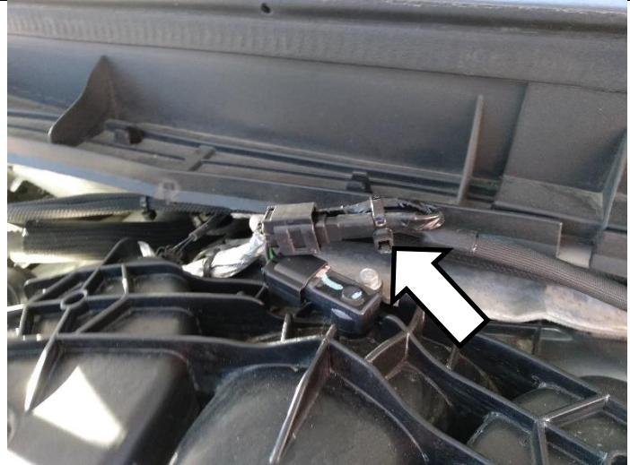
Install supplied zip-ties to support the wiring harness.
