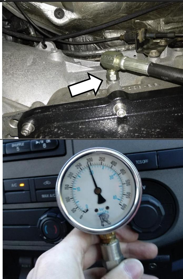
Stock pressure will range between approx. 70-170psi. With the BD kit installed the pressure is boosted up to 300 psi at higher engine load (15 psi+ turbo boost).
