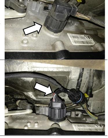
Route the supplied BD harness to the transmission and connect it inline.
