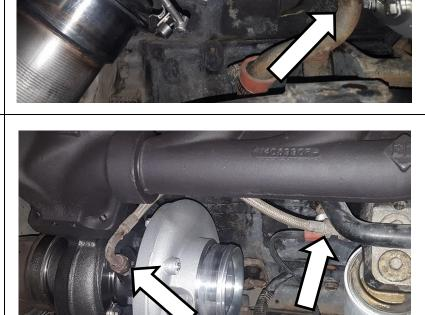
12.Connect the CAC pipe and boot to the turbo charger. Tighten clamps.
