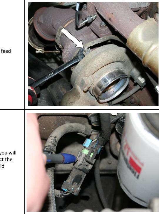
8. Remove turbo oil feed from the turbo.
