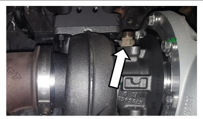
10.Install the supplied corrugated oil drain (Not shown in picture).Shape to fit. Ensure continuous down flow for the oil
