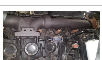
Install the BD Manifold using the supplied gaskets. 4. Install the coolant line bracket (1405998) as shown.
