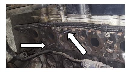
Install 4 supplied 25mm M10 studs onto the T4 flange. Use the 1/8NPT plugs to block the port on the manifold if not being used.
