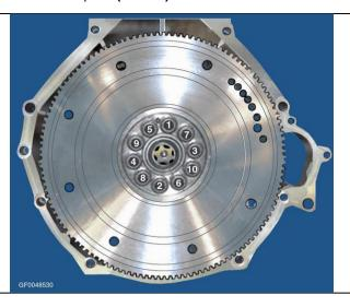
Lubricate the torque converter hub with multi-purpose grease, and re-install the transmission.
