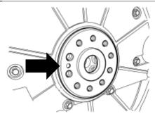
Install BD Diesel flexplate onto the crankshaft, followed by the washer.
