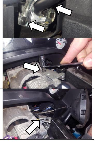
Take the shift lever over to a work bench with a vice. The next steps will involve transferring the new handle (5057438AC-P) into the original bracket.
