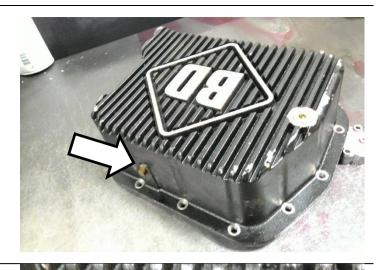
Feed the small end of the wire harness from the outside of the transmission pan to the inside.
