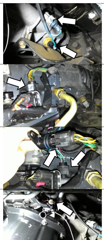
The BD transmission harness should be supported along the same route as the factory wiring harness and should be attached with wire ties to ensure it does not get near any moving parts and does not put significant strain on any of the wiring connectors.
