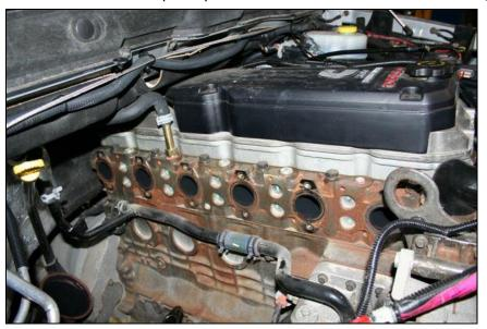
Install the 4 supplied studs (#1462430) into the manifold.
