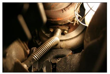
Using a cutoff wheel, cut the coolant line support bracket about 1-1.5" from the coolant tube. Leave enough material to re-connect the new supplied bracket to this tab.
