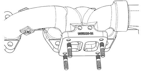
Now install your custom T4 turbo of choice, use the low-profile flange nuts to secure your installation (#1462441).
