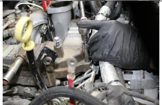
17. Remove the heat shield on the exhaust up-pipe. Remove the bolt holding the large coolant line next to the up-pipe and the two vertical bolts on the control valve (pictured).
