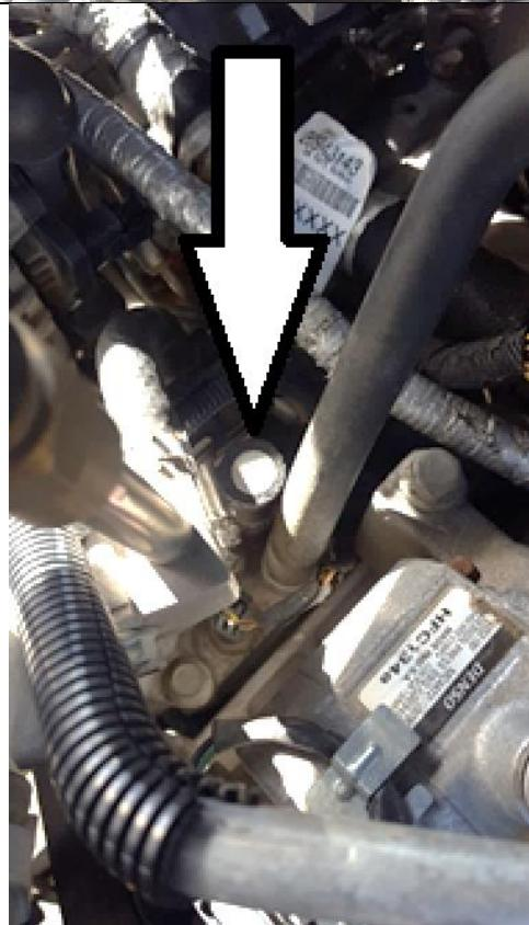
6. Plug the coolant hard line near the fuel filter as shown. Use the 5/16" plug (1462121), two spring clamps (1407153) and 2.5" of silicone line (1407155).
