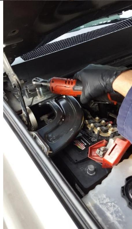
5. Disconnect MAF and humidity sensors from the intake.
