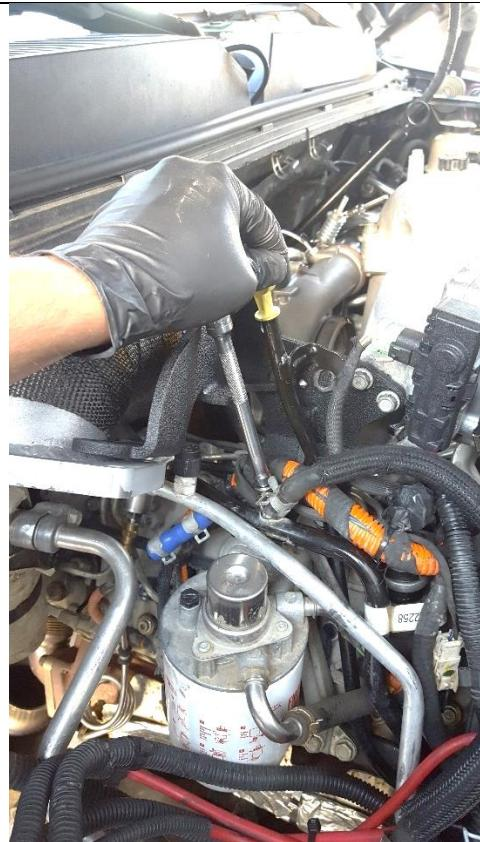
17. Use the supplied T6 gasket (2495146) and sandwich the turbo bracket, hot pipe, and turbine housing together as shown. Use the M10 socket head bolts (FT-35574) with the supplied 10mm nuts (1462441). Make sure the hot pipe sits snugly to the stock turbo and tighten everything into place.
