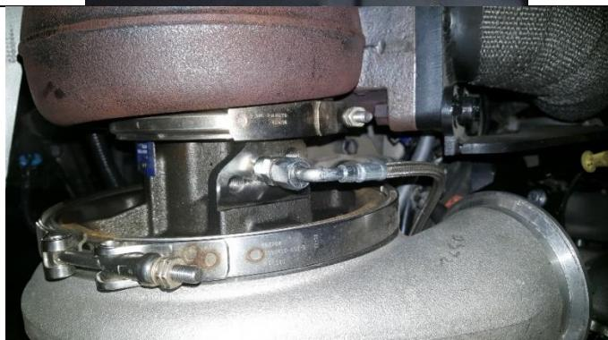
24. The secondary turbo inlet and primary turbo outlet need to be installed at the same time. Be sure to install the supplied #242 O-ring (FT-0480826) into the inlet flange. You may need to fully undo the OEM gear v-band clamp on the stock turbo to install the tube.
