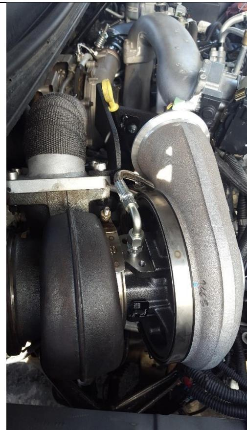
23. Pre-lube the primary turbo and install the oil feed line.
