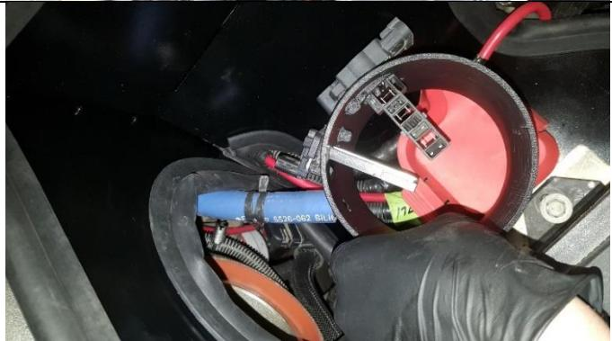
40. Push the intake tube through the air box aligning it with the 5" intake boot.
