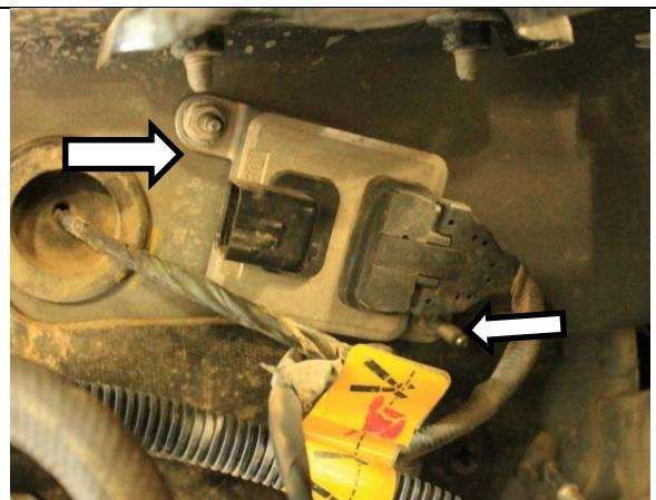
22. Remove the indirect fuel injector in the downpipe.
