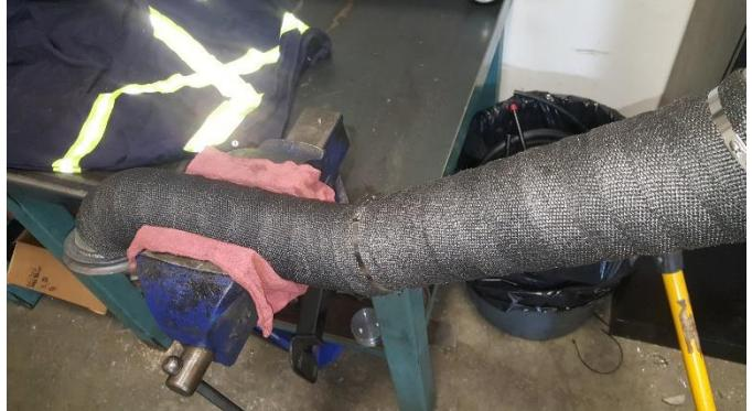
43. Twist the downpipe into place through the bottom. You should not need to force anything.
