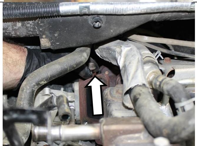
18. Lift the cooler assembly to access and remove four bolts securing the front cooler to the rear cooler.
