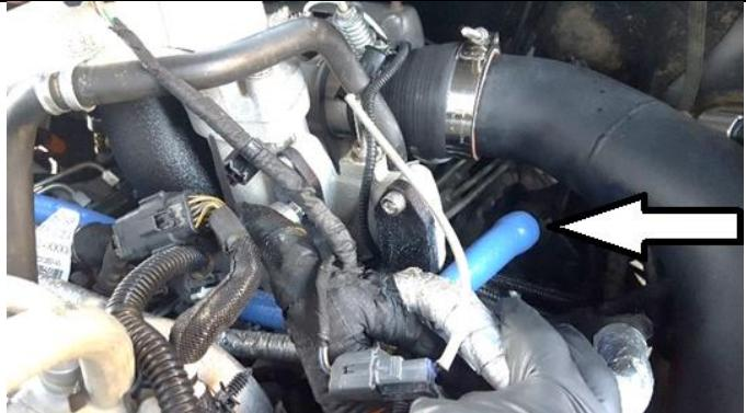
39. Connect the PCV tube and humidity sensors to the intake tube before pushing through the air box. Cut the PCV tube to length.
