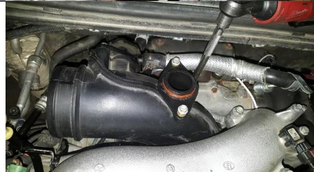
8. Remove the stock turbo intake tube. Completely loosen off the inlet gear clamp. Remove the PCV tube and attached P-clamp.
