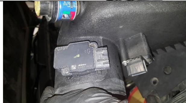
6. Undo the Philips head screws and gear clamps on the intake. Remove the stock air box and filter.
