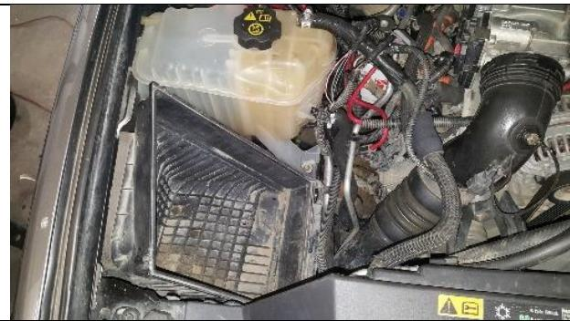
7. Remove the top two bolts with a 10mm socket and the front bracket with a 13mm socket. Remove the intake resonator.
