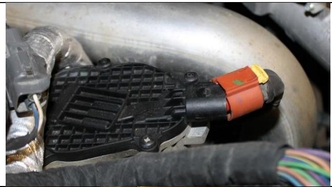
13. Unplug the control valve connector and remove all coolant lines connected to the recirculation (only 4 shown there are 5 in total to disconnect).
