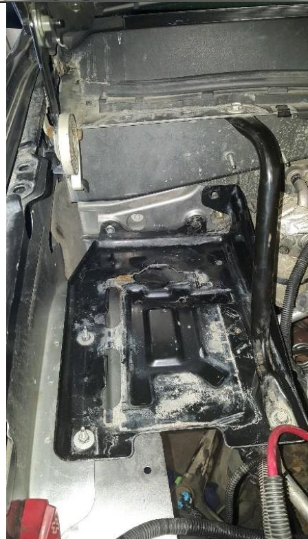
30. Two studs on the firewall will need to be ground off to clear the compound downpipe.
