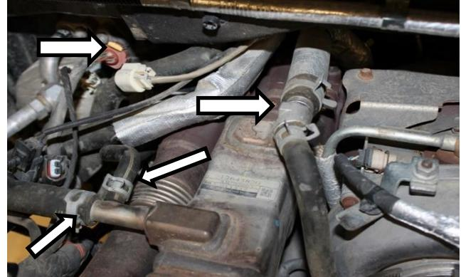
14. Remove the two bolts on the crossover tube on the passenger (by control valve) and driver (by recirculation valve) side.
