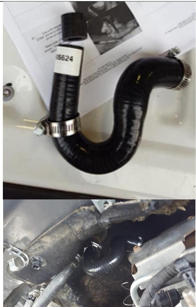
5. Plug the 1/2" coolant line near the front of the motor. Use the 1/2" plug (1462123) using 1/2" line (1604054) and two gear clamps (1453113).
