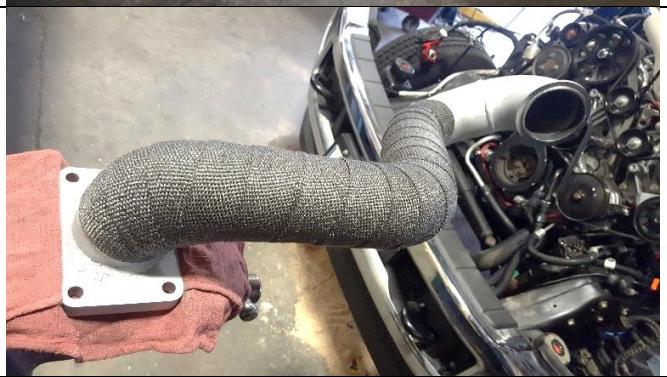
15. Use the stock downpipe v-band clamp and loosely clamp the hot pipe in place (1406612)
