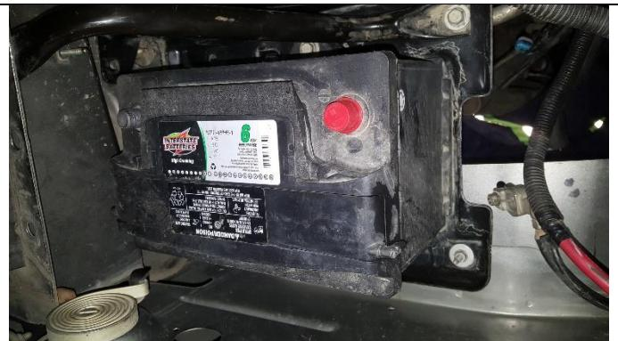
29. Remove the stock battery tray and brace. Do not lose the two 10mm head nuts on the fender.
