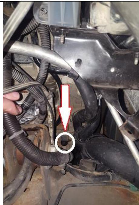
22. Install the  $\frac{1}{4}$ " NPT to JIC (1453162) fitting into the turbo CHRA. Make sure the oil inlet to the turbo is vertical.
