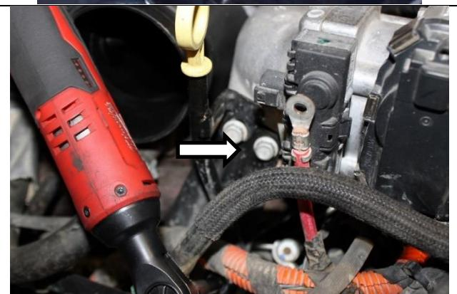
12. Unplug the orange connector on the recirculation valve.
