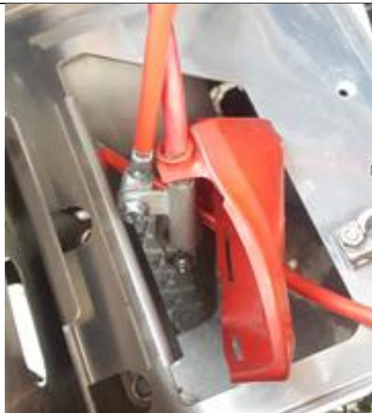
32. Install the weather stripping (1453820) on the air box as shown. Be sure to install weather stripping to protect the battery cables.
