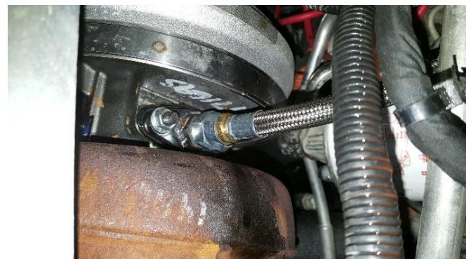
21. Unbolt the oil plug located in the block with a 17mm wrench. Install the ORB to JIC straight fitting (PN 1462323) and braided oil feed line (PN 1462329).
