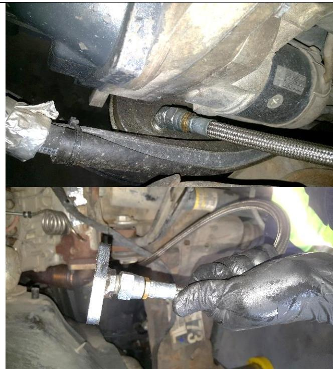
20. Install the turbo into the turbine housing. Ensure the turbo compressor wheel spins freely before tightening the turbine housing clamp. **Physical damage is not covered under warranty.**
