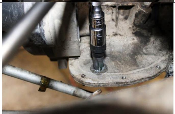
12. Use thread sealant and seal the 45 degree NPT to JIC fitting (FT-421680). Do not put sealant on the JIC threads.
