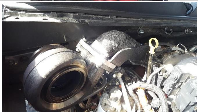
18. Secure the oil dipstick bracket to the primary turbo bracket using the M8 (FT-11116243) bolt.
