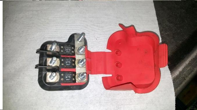
35. Pull the wires through the air box and connect the wires as per the diagram below. Make sure the fuse holder cover is secured in place after attaching all wiring.
