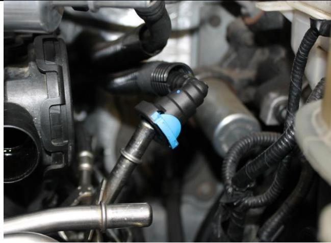
58. Install second quick-disconnect adapter onto return outlet (arrow 2). Apply FT-0606434 Loctite to 1500720 retaining collar (arrow 1), and slide over outlet, behind shoulder, and thread into adapter. Torque to 10 ft-lbs.
