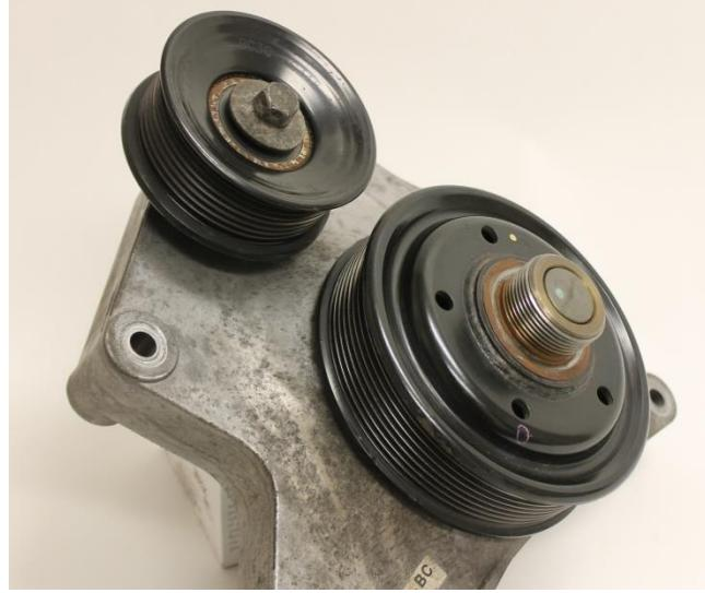
14. Using 13mm socket, remove fan pulley hub from front of engine.
