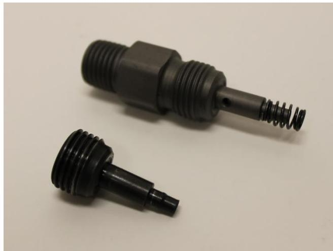
21. Install new output fitting with spring and ball bearing. Torque to 56 ft-lbs, using a 17mm socket.
