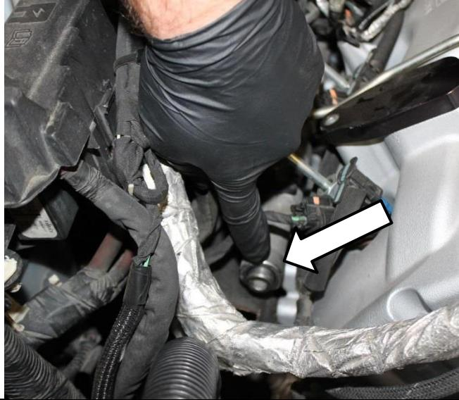
31. Install supplied fuel rail fitting 1500704, into previously plugged port (front end of passenger side fuel rail). Using a 22mm socket, torque to 75 ft-lbs.
