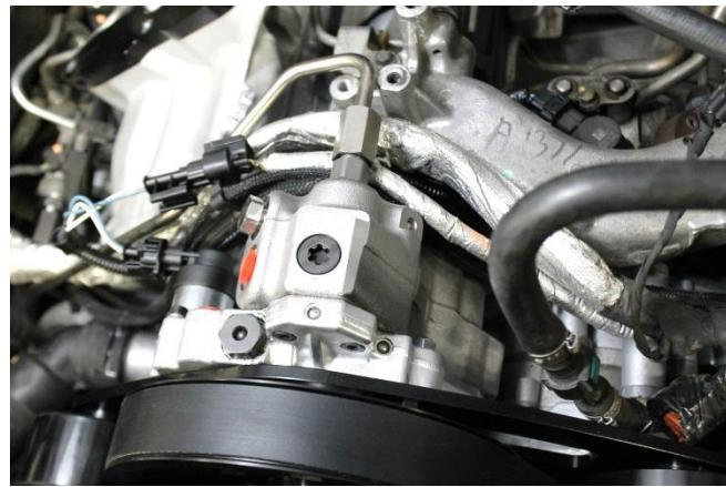
37. Remove the OEM CP3 inlet fitting and transfer the sealing washer over to the new 1502040 HiFlow fitting as shown.
