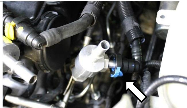
Insert 1500723 quick-disconnect fitting into end of supplied 1/2in fuel hose, and secure with 1452821 gear clamp.
