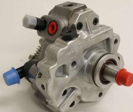
18. Using 17mm socket, remove OEM output fitting (seen here in black) from port. In its place, install plug 1500718 using a 17mm socket. Torque plug to 74 ft-lbs.
