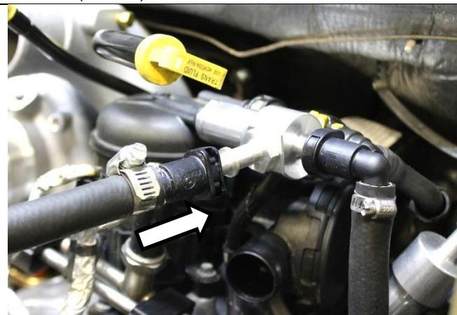
60. Trim to length and push hose over feed fitting on CP3 pump. Secure with 1452821 gear clamp.
