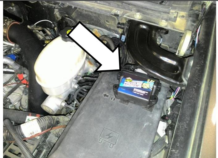
To check operation of the pressure controller, attach a mechanical pressure gauge to the Allison transmission test port. Whenever the truck is over 15 psi of boost the line pressure should go to maximum (250-275psi).
