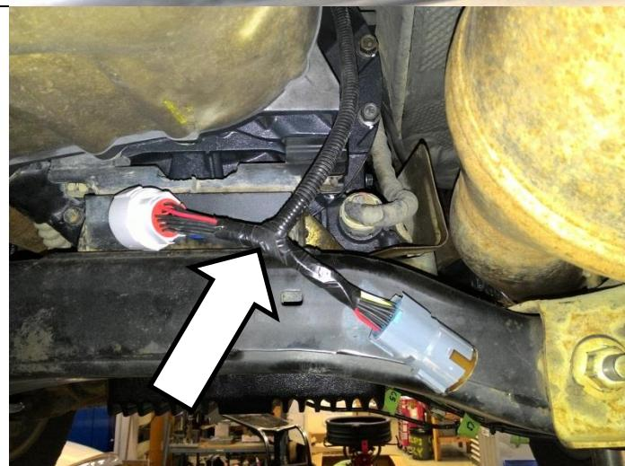
Disconnect the transmission 20 way round electrical connector by squeezing on both sides and wiggling it off. You may either use the special Allison tool for this, long needlenose pliers or remove the heat shield to get your fingers on the connector.
