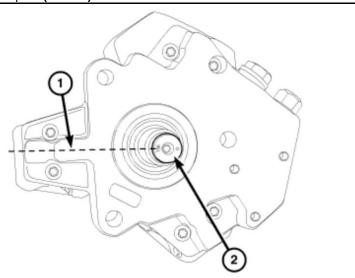
Position injection pump to mounting flange on gear housing while aligning injection pump shaft through back of injection pump gear. Be sure the "line" is still at the 9 o'clock position (1).
