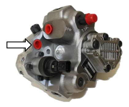
Install fuel line (injection pump-to-fuel rail). Note with the BD High Performance pump you may need to tweak/bend the factory high pressure line.
