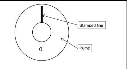
Rotate the injection pump shaft until the "line" is positioned at 9 o'clock (1).
