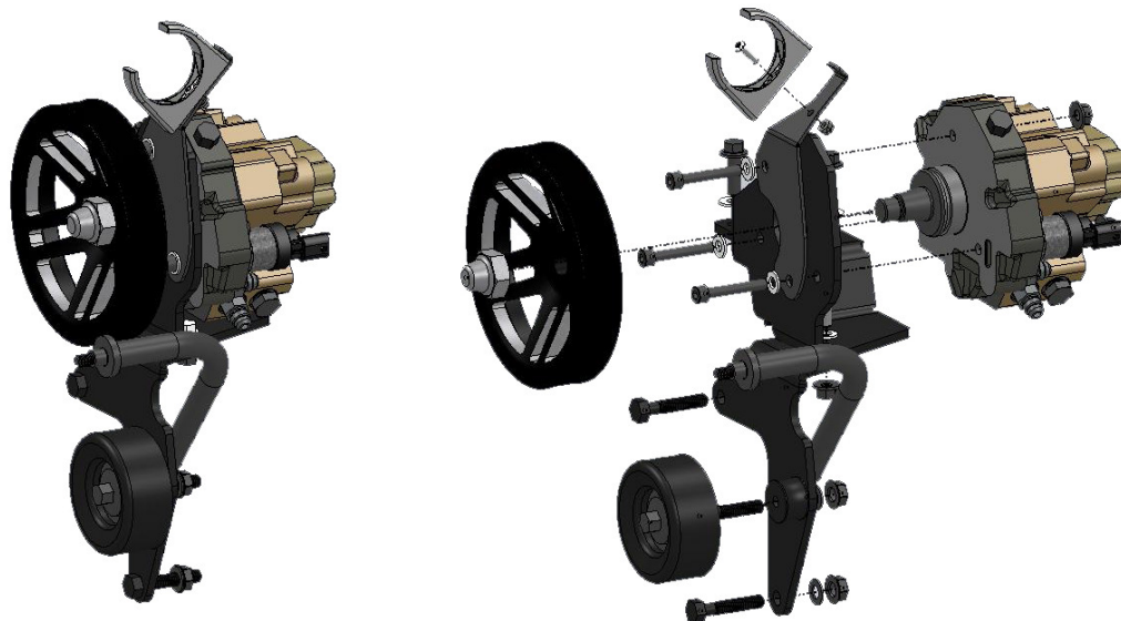
Figure 8 - Pump Mounting and Bracket Assembly
