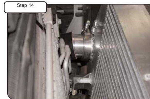
Position and make sure intercooler rubber U-shaped isolators sit square on cross beam and have not folded during installation.
