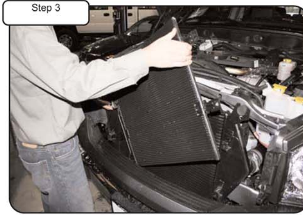
Step 3 Rotate the A/C condensor up and out away from vehicle. Take care to prevent damage to A/C lines.
