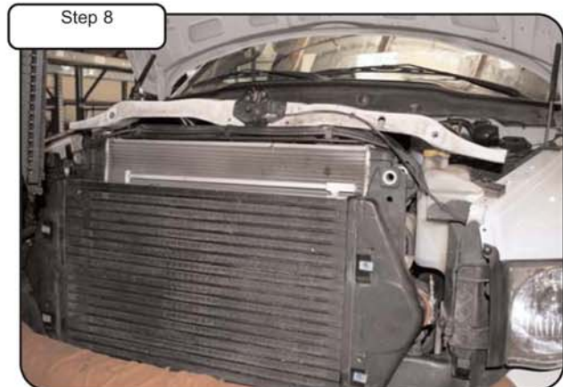
Step 8 Remove the upper radiator support and set aside on top of fan shroud.
