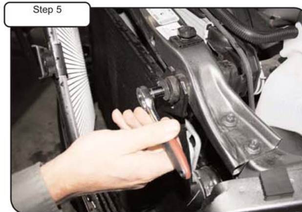
Step 5 With 10mm socket or wrench remove the 2 top intercooler attachment bolts connected to upper radiator support.
