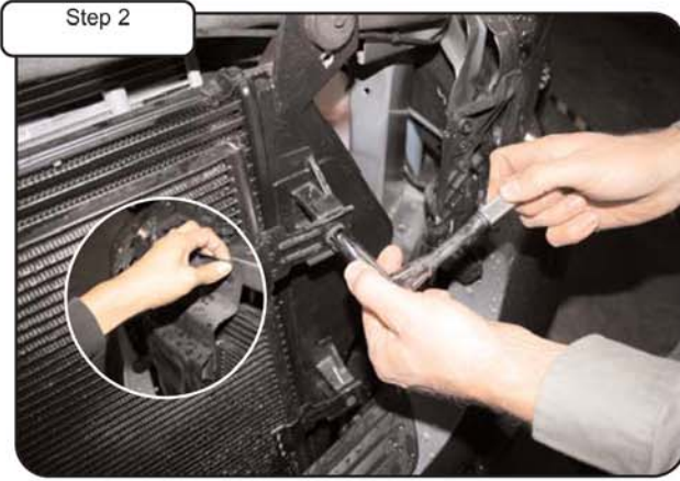
Step 2 Remove plastic A/C line protector on passenger side. With 13mm socket or wrench. Now loosen the 4 bolts holding in A/C condensor.
