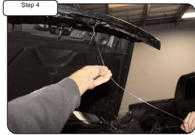
Step 4 With A/C condensor turned 90 degrees, secure to the vehicles lifted hood using steel wire.
