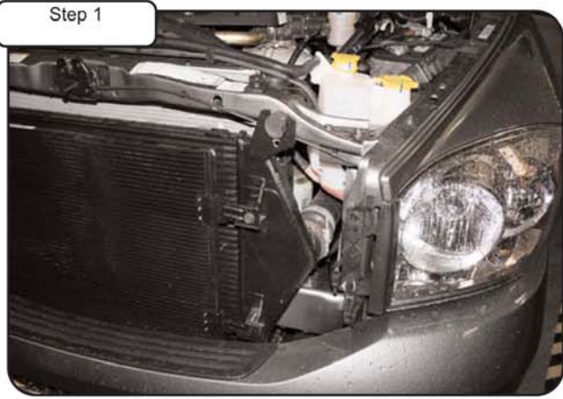
Step 1 Stock Intercooler. NOTE: Disconnect battery before install. Remove stock air box or intake system from vehicle for easier installation.
