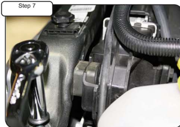
Step 7 Loosen and remove the 4 bolts holding in upper radiator support using 13mm socket or wrench.
