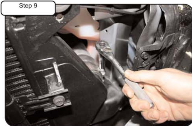
Loosen clamps on intercooler tubes using 7/16" deep socket.
