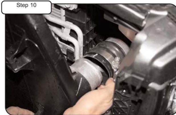
Pull back coupler from intercooler. Now remove stock intercooler out of vehicle.
