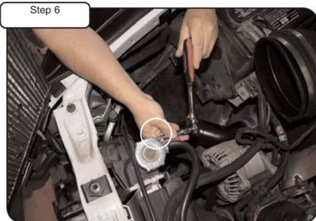
Step 6 With 10mm socket and extension loosen the two bolts holding in radiator on back of upper radiator support.
