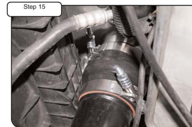
INTERCOOLER MAY NEED ALIGNMENT, TIGHTEN WHEN IN CORRECT POSITION & PROPER CLEARANCE. Re-install Radiator support (See reverse steps 5 through 8). Tighten and torque all clamps to 5 ft. lbs.
