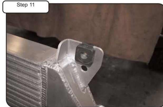
Remove the two upper-rubber isolators with spacers from stock intercooler and install to new BladeRunner® intercooler.
